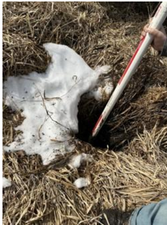
Tile blowout that was located on the system.
