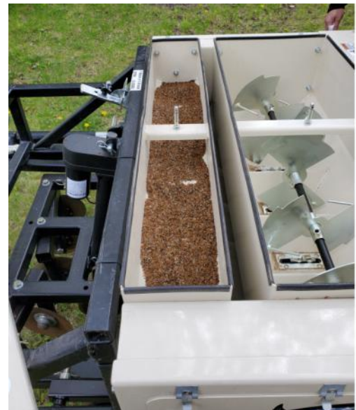
Above: Le Sueur SWCD using the Dew Drop Seeder to seed buffers. Below that is a photo of the inside of the small seed box on the Dew Drop Seeder.
